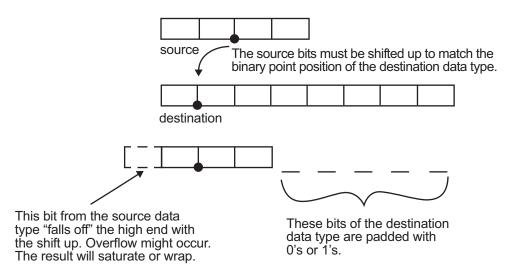
As the diagram shows, the source bits are shifted up so that the binary point matches the destination binary point position. The highest source bit does not fit, so overflow might occur and the result can saturate or wrap. The empty bits at the low end of the destination data type are padded with either 0's or 1's:
