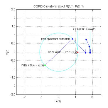
The second rotation is about the first and third row of R and the first and third column of Q. Element R(1,1) is the pivot and R(3,1) rotates to 0.
