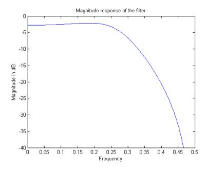
Notice that the high frequencies in the input signal are attenuated by the low-pass filter which is the expected behavior.
